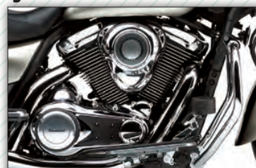
1,700 cm 3 , 50° V-Twin, Liquid-Cooled
