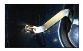
Remove the right rear trunk bolt and install the provided metal grounding bracket at this point and to the lower mounting hole of the antenna base.
