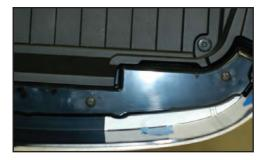
Carefully mark the center of the holes with a scribe and drill pilot holes from the inside of the trunk using a 1/16" bit. Finish drilling the holes from the outside using a 7mm (1/4") bit.
