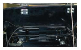
Cut the antenna base drilling template out of the instruction sheet. Carefully fold it at the score lines and tape to the inside right rear corner of the trunk as shown.
