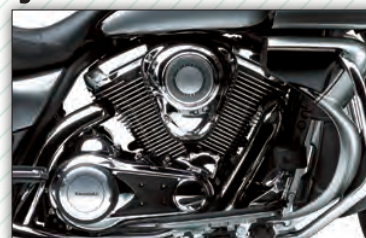
1,700 cm 3 , 50° V-Twin, Liquid-Cooled
