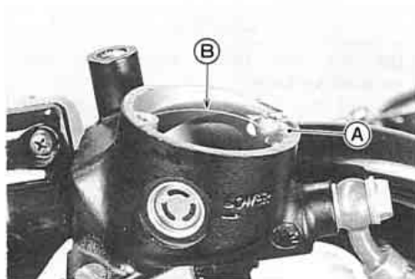
A. Front Brake Fluid Reservoir B. Upper Level Line
