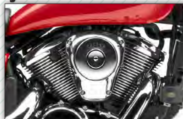
903 cm 3 , V-Twin, Liquid-Cooled Engine
